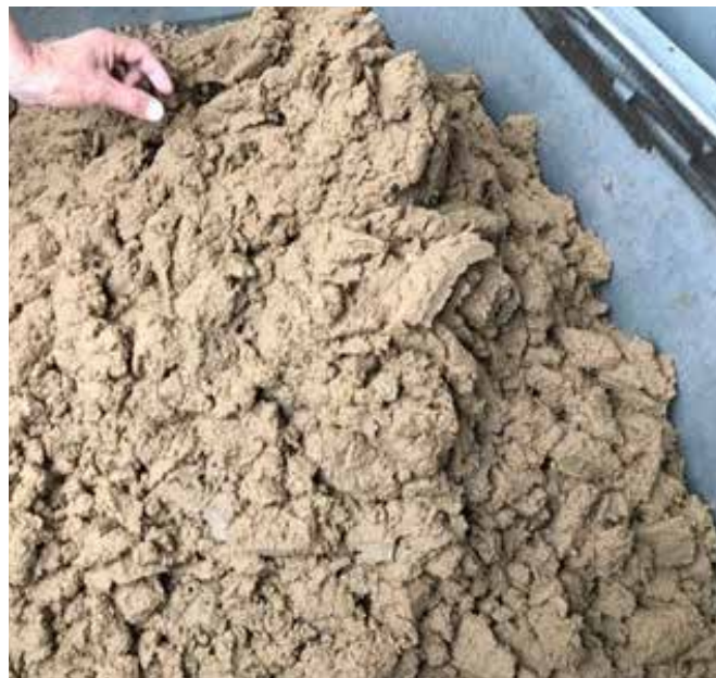
Lighter, drier, healthier and more easily recycled and transported dried sludge produced using KDS technology
