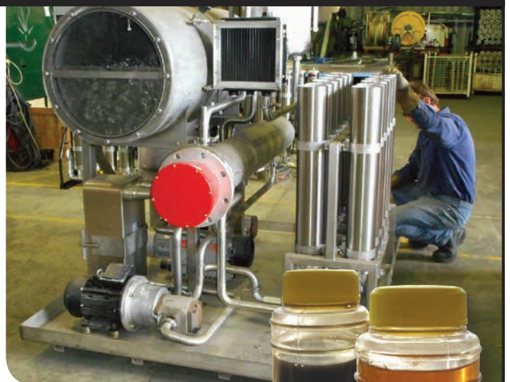
Filter Technology Vacuum Dehydrator/Filtration system undergoing final inspection at our Thornton manufacturing facility.
